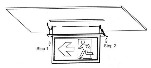
7, Rotate spring to up, press the fixture with recessed kit on mounting plate, press in one side then another.
