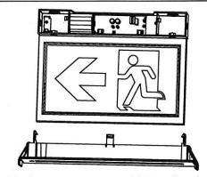
4, Assemble fixture on recessed kit, notice the direction of fixture.
