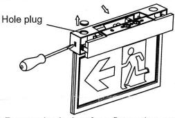
2, Remove back plate from fixture, then remove hole plug at test switch side.
