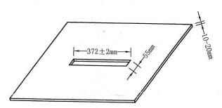
1, Make a cut out hole, dimension 372mm\*55mm. The thickness of mounting plate 10 to 20 mm.
